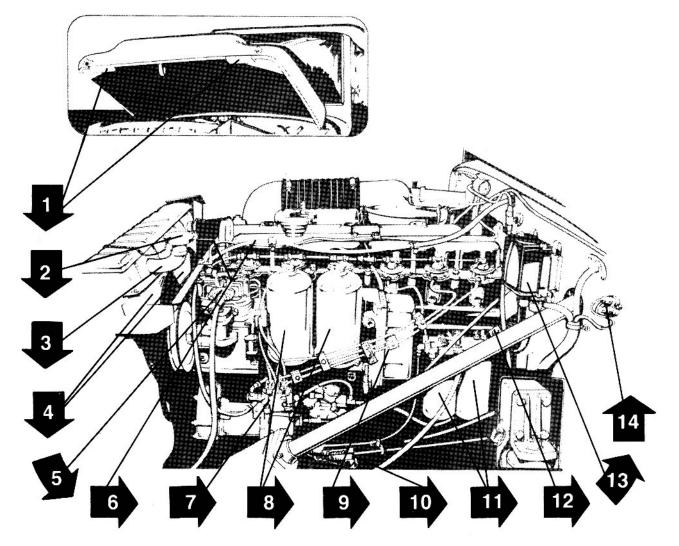
This Systematic Inspection Procedure is designed to make it easier for you to inspect and check your  $2\frac{1}{2}$  ton truck to help keep it "always ready" to move. Simply follow the direction of the arrows as you make your inspection.
